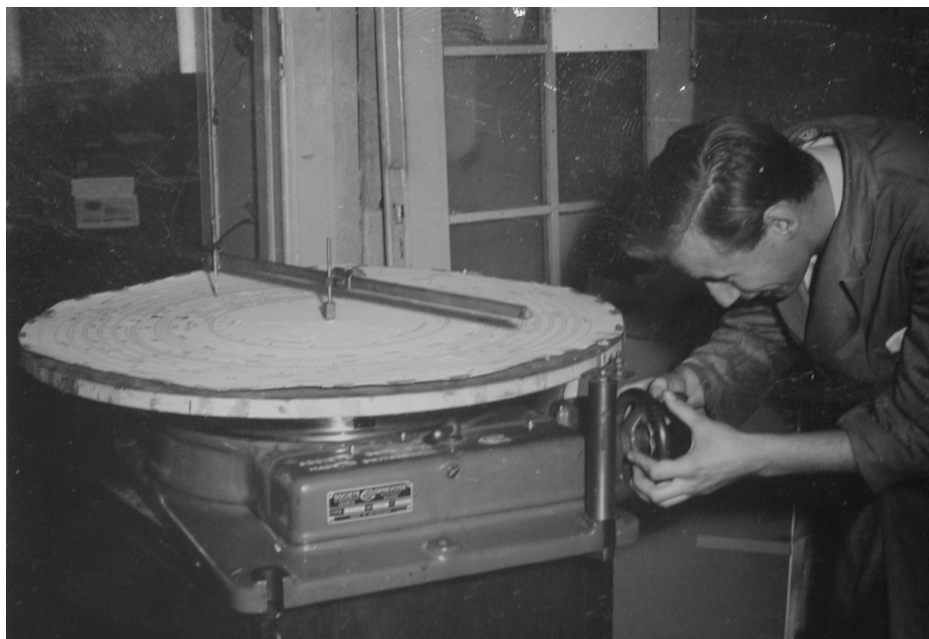
Figure: Production of scales for ALRO slide rule discs
