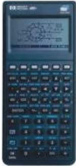
A new type of pocket calculator was introduced in the early 90's, the “graphical calculator”. This type has a somewhat larger screen display, to show not only calculation results, but also graphics of mathematical functions. The HP 48 was one of the first graphical calculators, but competing products were released by TI, Sharp, Casio and others.
